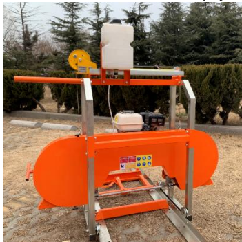
Correct head placement; Operators side is on side with the scale stick and hand winch.
