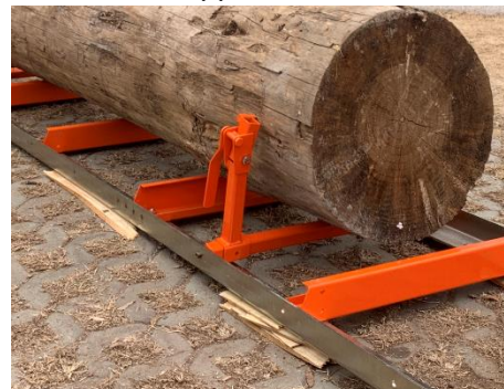
Squaring arm on left adjustable dog on right
